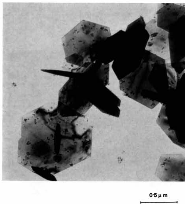
Fig. 1. Pyrrhotite hydrothermally synthesized from \text{Na}_2\text{S} and Mohr's salt solution at 200^\circ\text{C} . The small particles are mackinawite.
